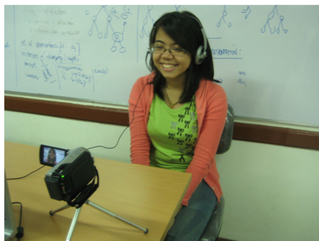
Figure 1. Data Collection Set-up. The subject is shown wearing a headset with a microphone, and a video camera that records the laughter episodes.
