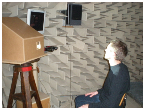
Figure 2: Recording setup: one speaker sits in front of the 3D scanner in the anechoic room while watching a video for instructions on the screen.
