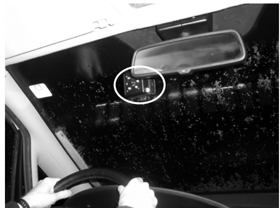
Figure 3: Camera position besides the rear mirror.
